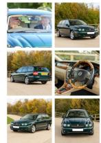
The Jaguar X-Type is a front-engine, all-wheel/front-wheel drive compact executive car manufactured and marketed from 2001 to 2009. In addition to offering Jaguar's first estate in series production, the X-Type would ultimately introduce its first diesel engine, four-cylinder engine and front-wheel drive configuration.
