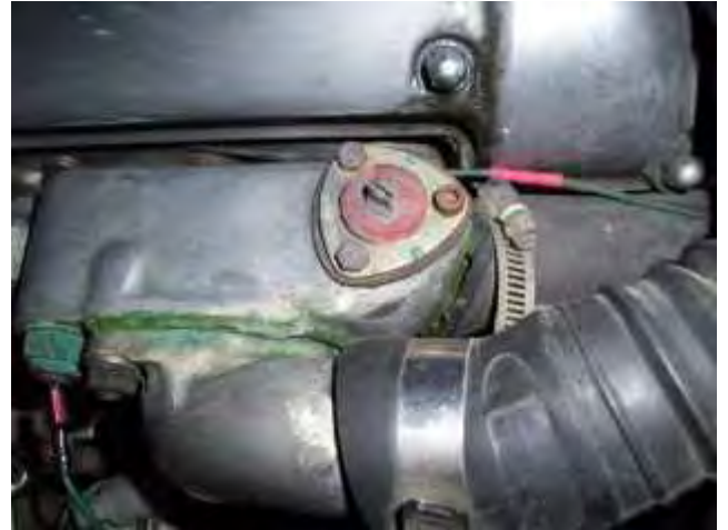
The Otter Switch is the rounded device with the red insulator. This car has been modified to manual control.
